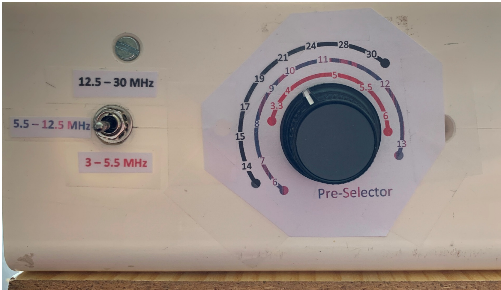
Figure 3. Band select and Pre-selector.
