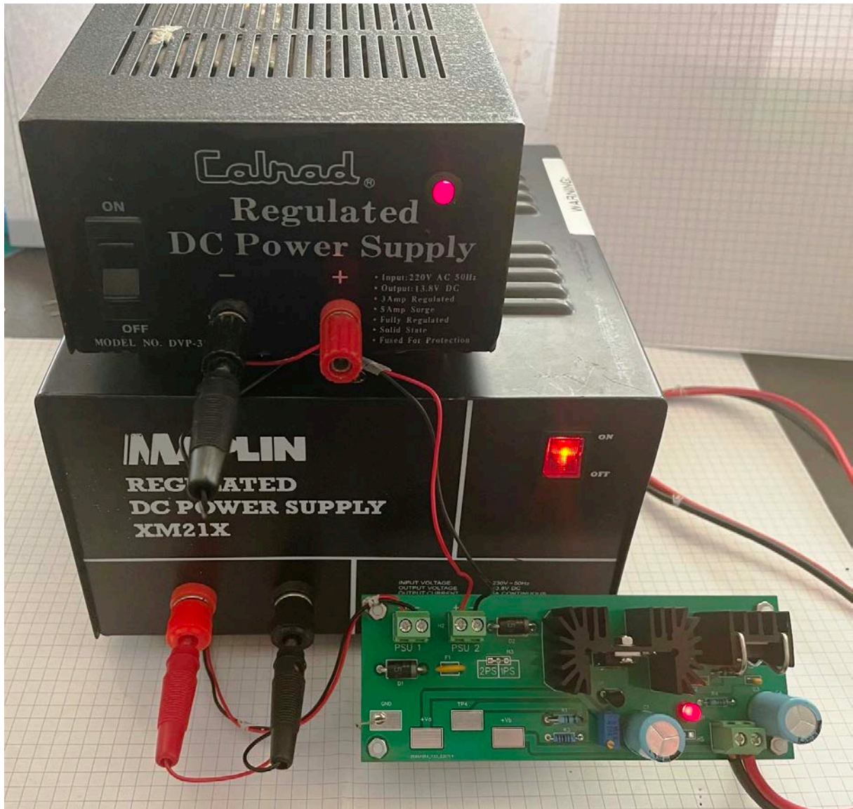
Figure 9. Using two fixed power supplies in series.
