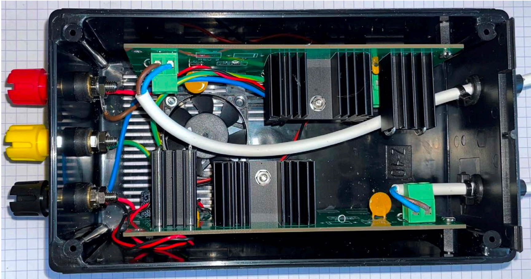
Figure 10. Inside the dual power supply enclosure.
