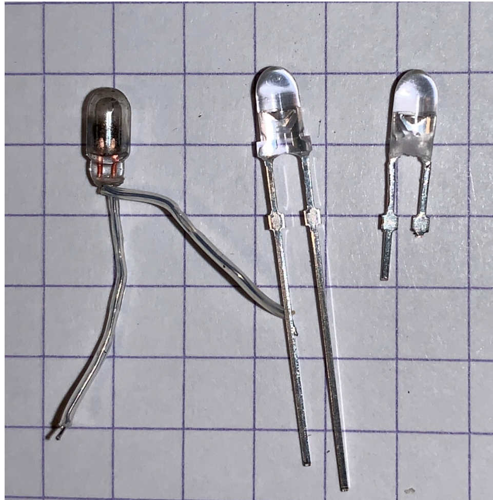
Figure 5 – Comparing the bulb, an untouched LED and a cropped and filed down LED
